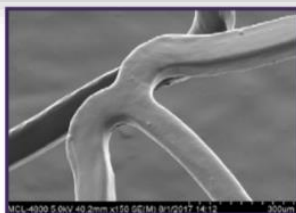
XIENCE Sierra (3.5 x 18 mm) 150x magnification at max expansion of 5.5 mm
